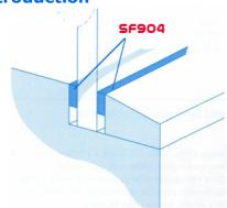
Sealflex **SF904** is a clean, simple and effective non load-bearing sealant medium that will prevent ingress of water, air and noise into a joint structure. The butyl based tape includes modifiers that will cause the material to intumesce at elevated temperatures resisting the spread of fire and toxic gases through the joint.
