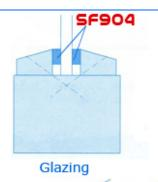
Typical glazed section, as tested by Trada Technology Ltd.
