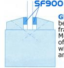
Glazing - Non loadbearing seal between frame and glass. Meets requirements of NHBC & BS6262 when used as part of an approved system.
